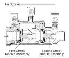
The 007 Series features a modular design concept which facilitates complete maintenance and assembly by retaining the spring load.
