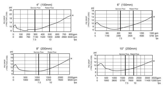
Flow capacity chart identifies valve performance based upon rated water velocity up to 25fps
